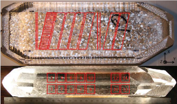
Figure 1 : Quartz crystal resonators according to their positions in the mother block.
