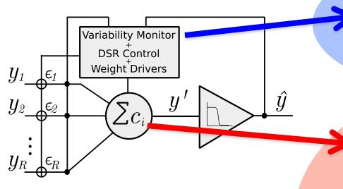
Variability Monitor based on a disagreement detector between the AD-AVG output  $\hat{y}$  and the signal provided by each replica  $y_i$
