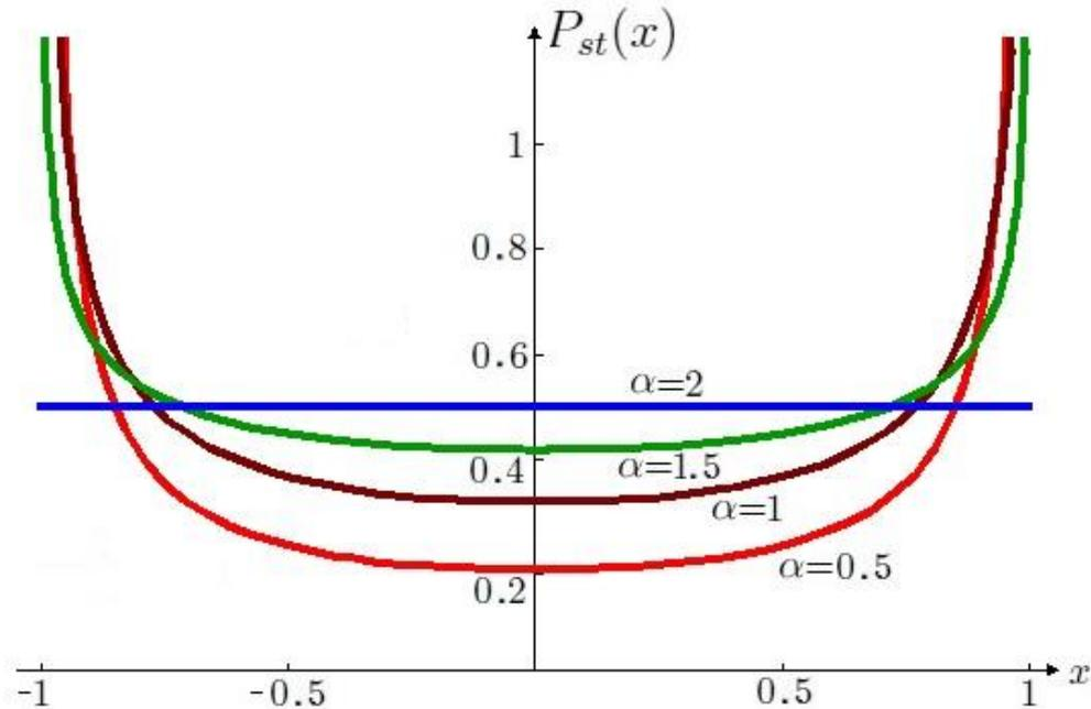
Plots of stationary probability density for different values of the Lévy index . The value of the parameter  $L = 1$ . The case  $\alpha = 2$  corresponds to usual Brownian motion.
